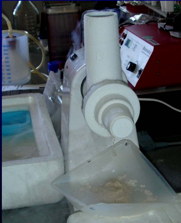
Liquid nitrogen cooled wheat mill in Küpper lab
